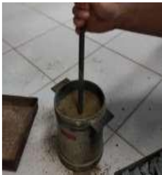
Figure 4. Bulk Density Testing Process of Fine Aggregate
