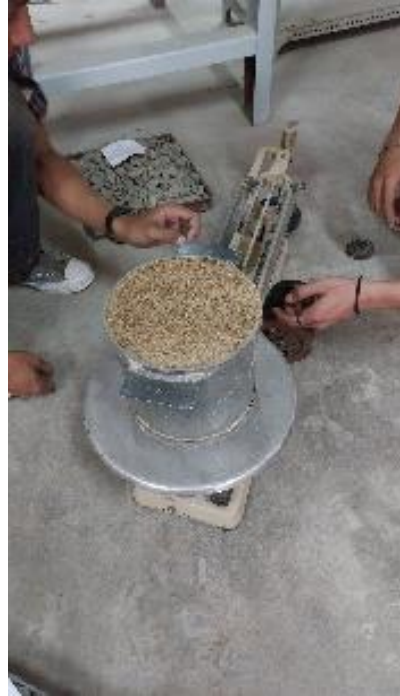
Figure 2. Moisture Content Testing Process of Fine Aggregate (Oven Drying Method)
