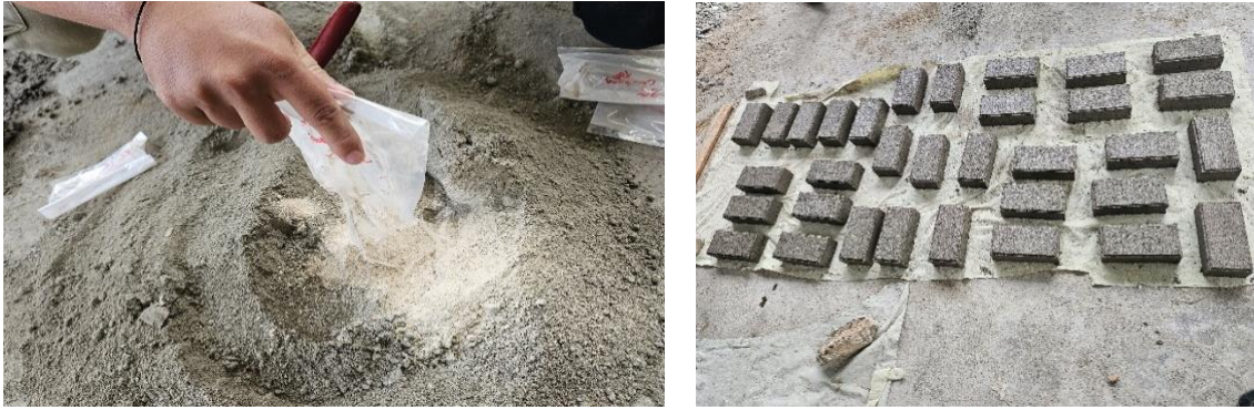
Figure 6. Mixing Process of Eggshell and Green Mussel Shell Ash into the Paving Block Mixture
