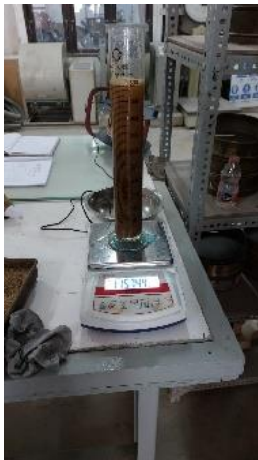
Figure 3. Specific Gravity Testing Process of Fine Aggregate
