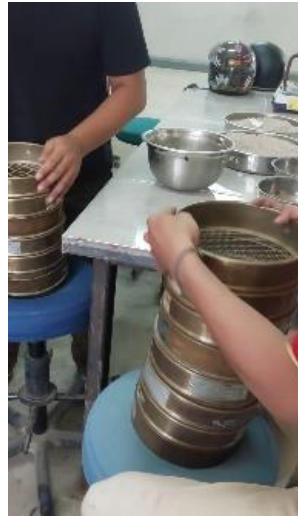
Figure 5. Fine Aggregate Sieving Process
