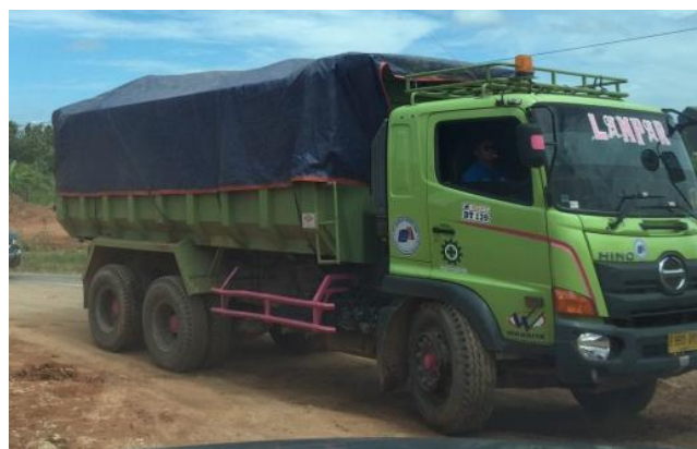
Figure 1. Covering construction materials.
